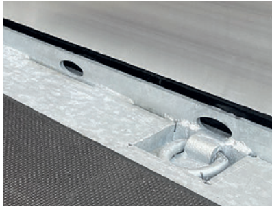
Safety Lock multi-point load securing system.
