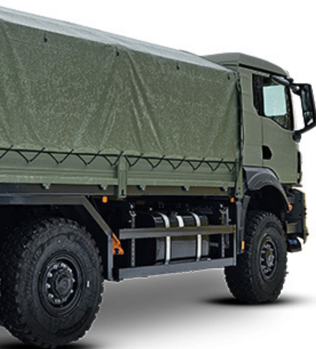
Tarpaulin made of hardly flammable or non-flammable materials
